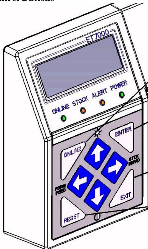
ONLINE - Used to toggle the Unit's operating state between "online" (ready) to "offline" (standby). Pressing this button while in the menu system causes the Unit to return directly to the "online" state.
